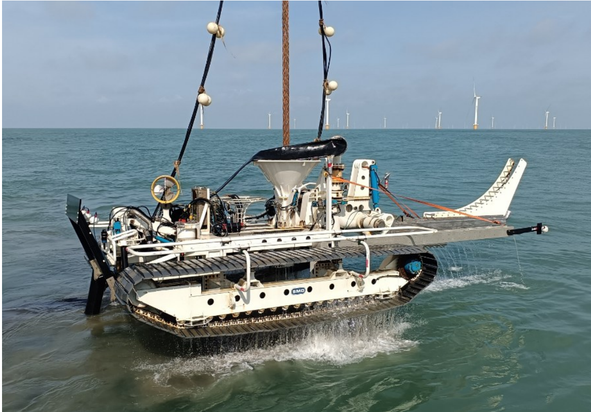
Figure 3.13 Shallow water trencher (source: https://www.smd.co.uk/blog/may-2023-smds-shallow-water-trencher-the-story-so-far/ )
