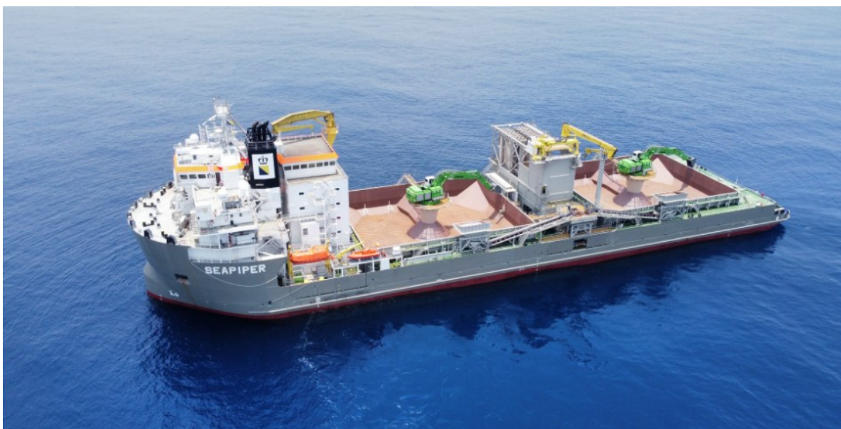
Figure 3.8 Example of a fallpipe vessel (source: https://www.portalmorski.pl/zegluga/53382-nowy-podsypkowiec-boskalisa )
